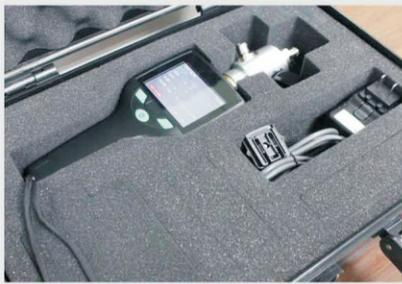
Models with optional portable dew-point monitor is convenient to test dew-point temperature of different machines.
